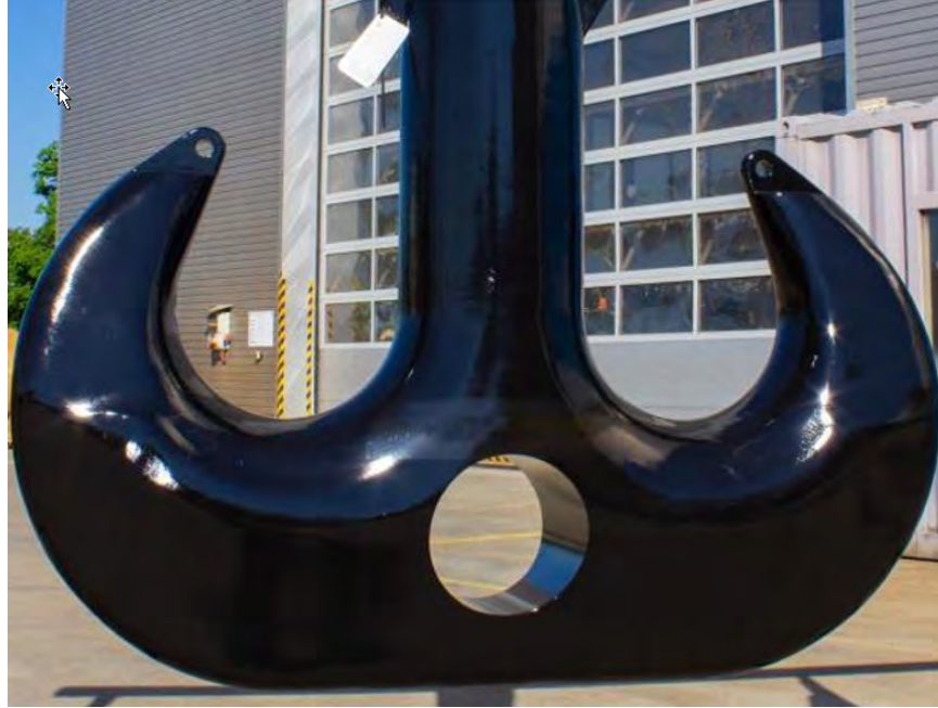
Figure 7. A crane hook capable of lifting of 350 metric tons was manufactured entirely using DED-WAM. The hook measures 3ft by 4ft and weighs 3,800lbs. 13
