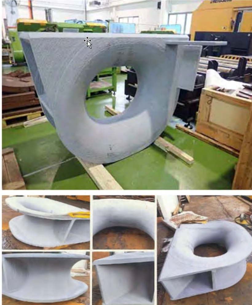
Figure 6. A 3200 lb. Panama Chock was manufactured using DED-WAM (wire). This part replaces a casting. 12
