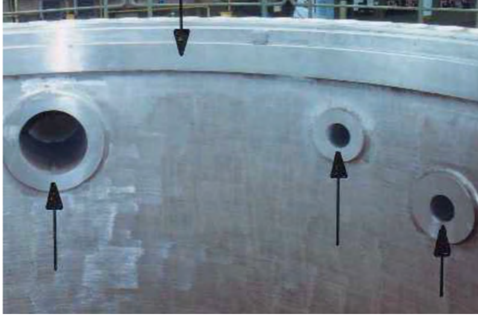
Figure 8. This photograph shows nozzle opening reinforcement and flange surfaces in the Atucha 2 reactor vessel in Argentina 17 . The circular features were created in place by Siemens using DED-WAM.
