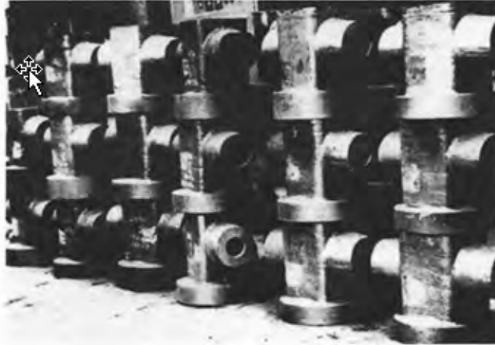
Figure 1. Electroslag castings of stop valve bodies 2
