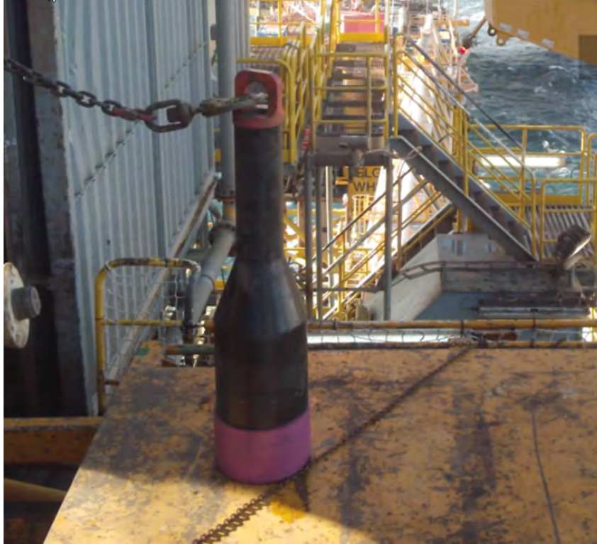
Figure 4. Water Bushing. A high-strength steel water bushing weighting 485 lbs. and nearly 4ft tall was manufactured using DED-WAM (wire). 10
