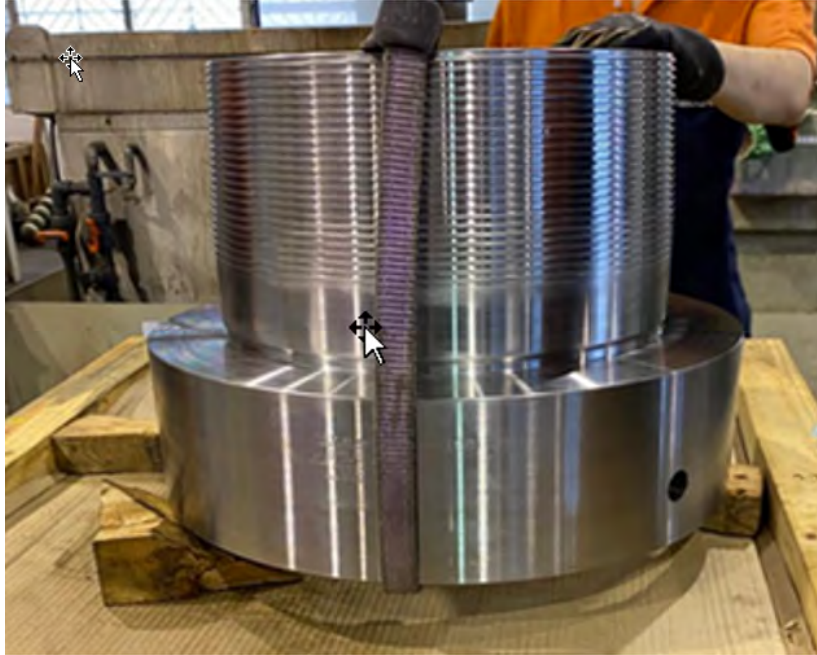
Figure 5. A 385lb lifting plug that is designed to lift a full drill string of over 100-tons at an off-shore oil rig in the Timor Sea. The lifting plug was manufactured using DED-WAM (wire). 11
