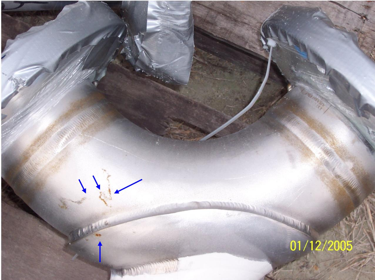
The photograph shows rust on a stainless steel pipe spool piece.
