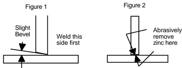
The welding engineer should also check the welding electrodes which are being used for high silicon levels. Excessive silicon can cause zinc to penetrate the weld metal, leading to cracking, especially when the zinc coating is thick. The silicon in welding electrodes should not exceed 0.85%; this means that commonly used ER70S-6 filler metals should not be used when welding galvanized steel.
